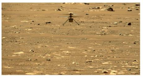
NASA's Mars Ingenuity drone survived a close call that could have ended in disaster. During its sixth flight, a glitch in its camera image delivery pipeline caused the drone's onboard navigation system to malfunction.
